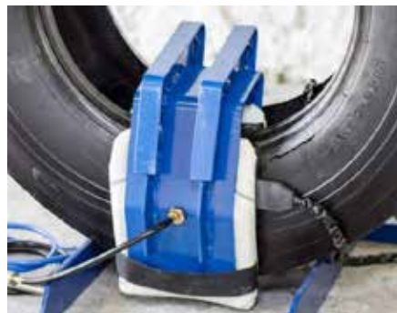
Truck/OTR/Agric Sidewall repair
