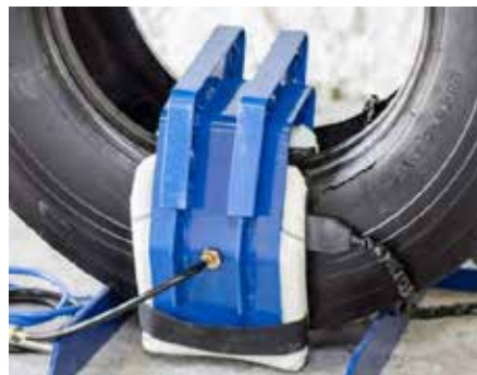
Truck/OTR/Agric Sidewall repair
