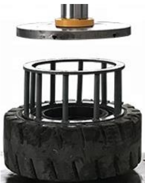
Forklift Solid tyre fitment
